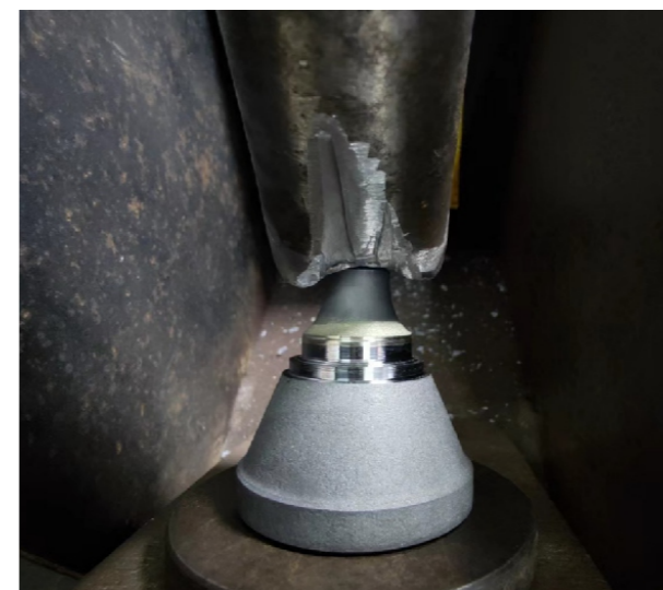
Random sampling inspection Professional testing equipment to test weld strength
