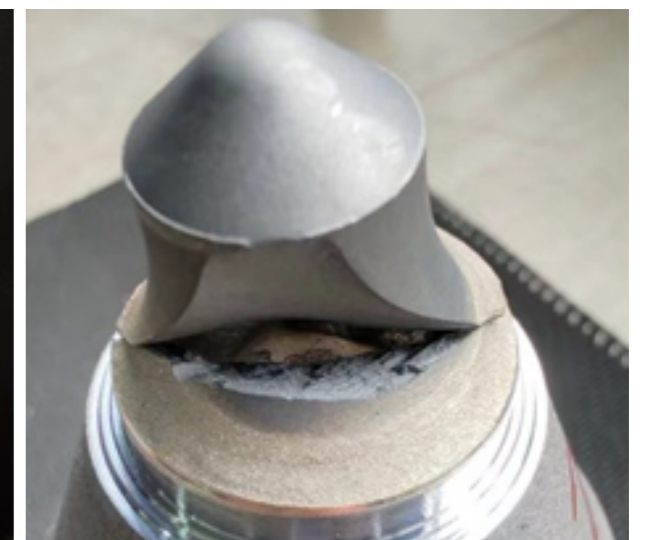
Destructive test result The weld joint is firm and not falling off
